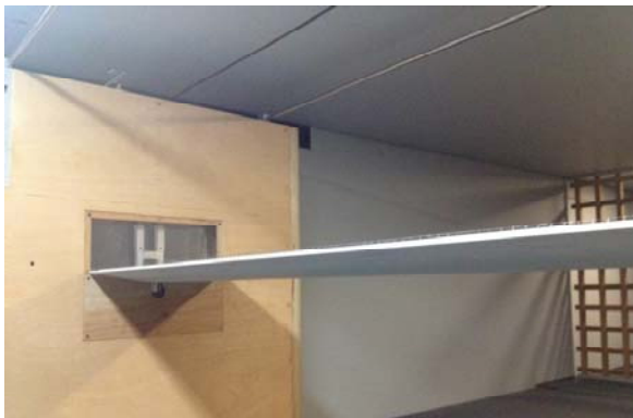
Deck model scale 1/150
