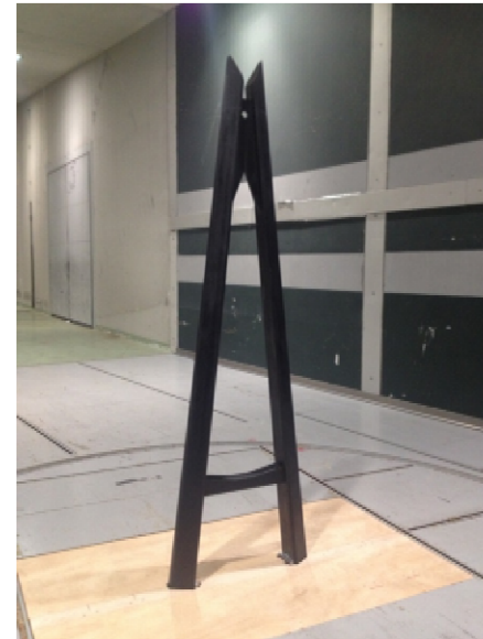
Rigid tower model (scale 1/150)
